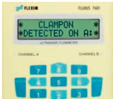
Plug & Play transducer identification
